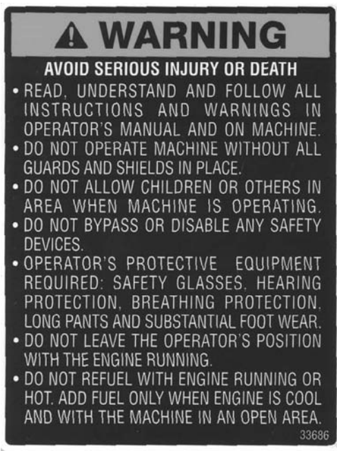
7033686 - LEAF BLOWER WARNING - LOCATED ON SIDE OF BLOWER HOUSING
