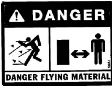
7033874 - DANGER-FLYING MATERIAL - LOCATED ON SIDE OF BLOWER HOUSING
