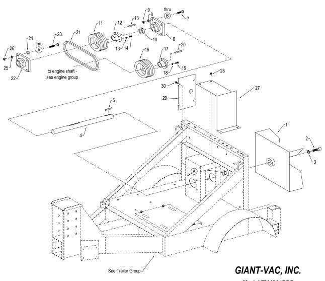
Model TM4201PDB Sheet 3 of 6 Impeller Drive Group R0603.1
